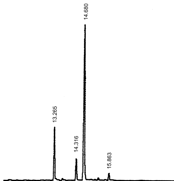
Figure 1. Capillary GC analysis of gas-phase thermal reaction mixture from 1 (without internal standard) after 6.5 h at 315 °C: 2 , 3 , 1 , and 12 (from left to right).
